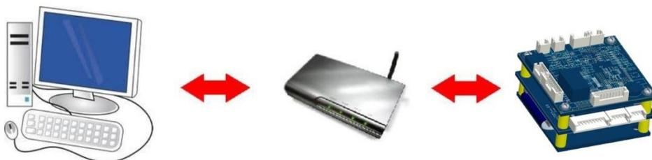
To connect the IP Camera to a network via a Router:
