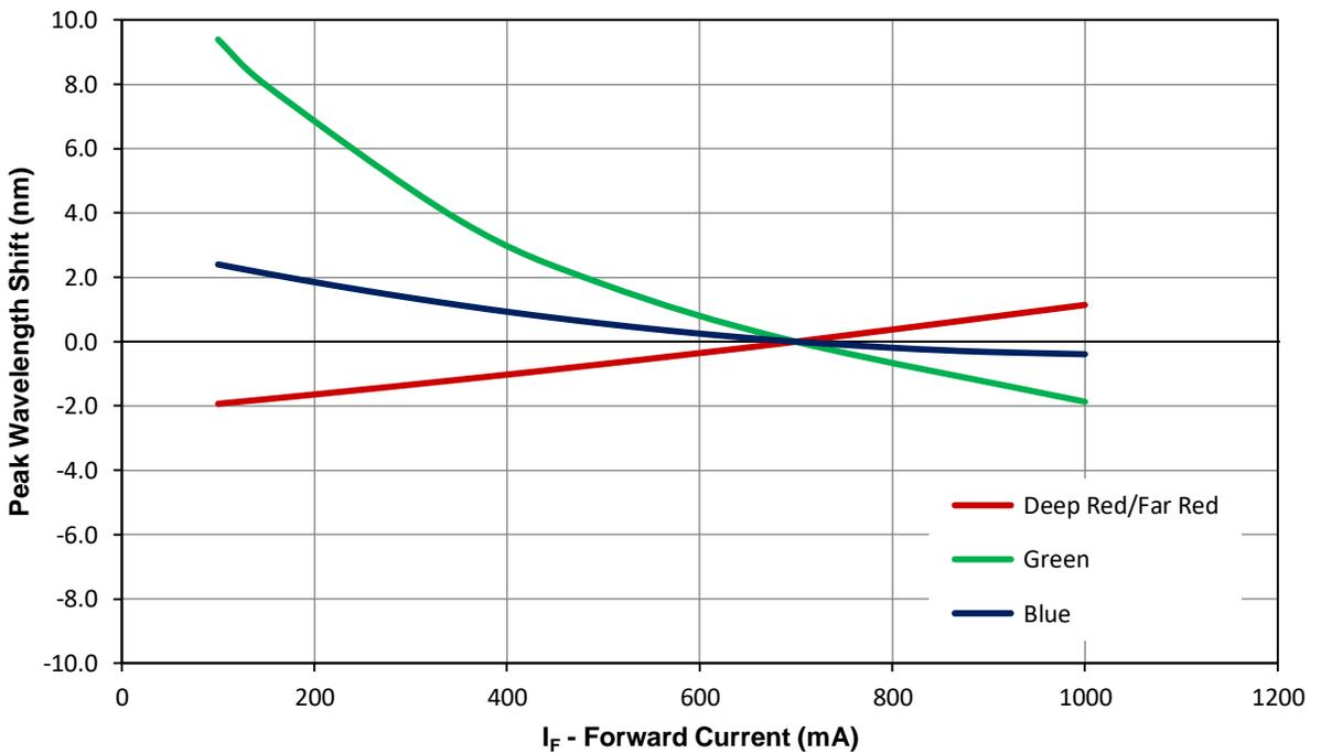
Figure 9: Typical peak wavelength shift vs. forward current @ T<sub>C</sub> = 25°C
