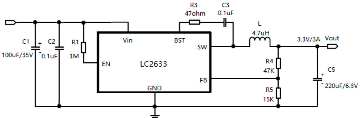
C<sub>IN</sub> & C<sub>OUT</sub> use electrolytic capacitors application circuit
