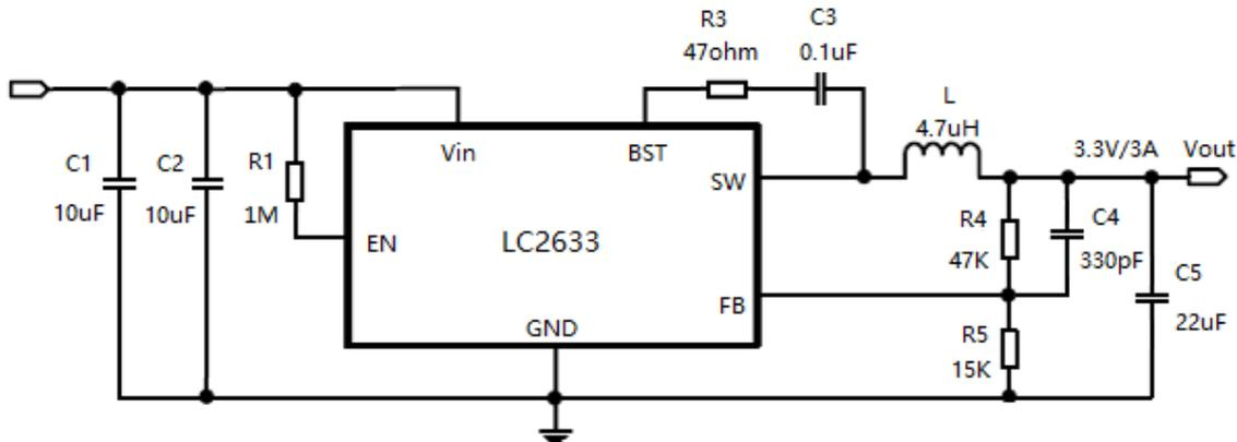
C<sub>IN</sub> & C<sub>OUT</sub> use ceramic capacitors application circuit
