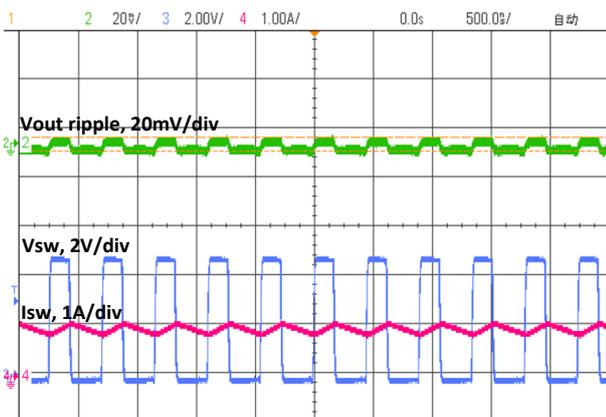
**Output Ripple and SW at 1A load**
