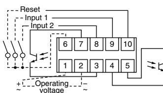
Note) For connecting the output leads of the transistor output type, refer to 5) Transistor output on page 141.
