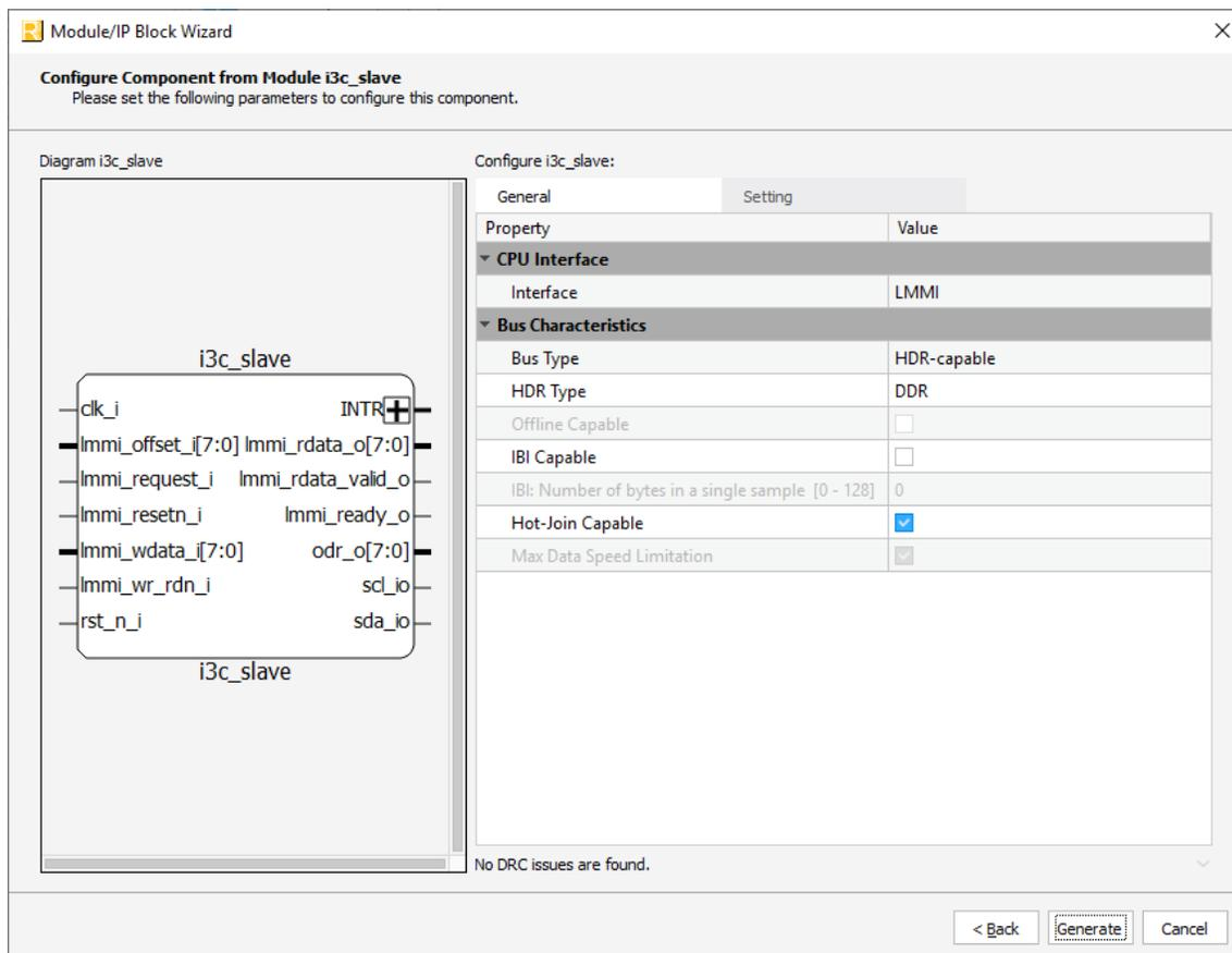
Figure 3.1. Configure Block of I3C Slave Module
