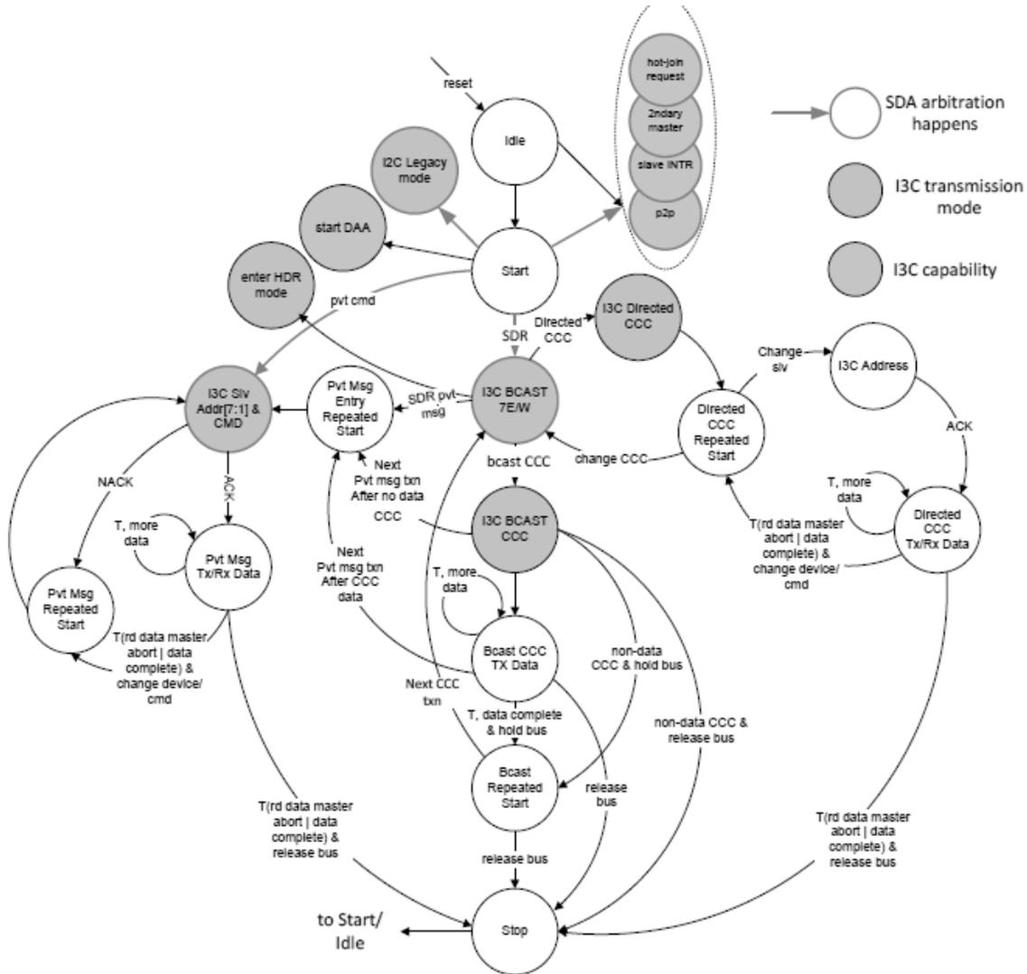
Figure 2.4. I3C Main Master Key Transmission Modes
