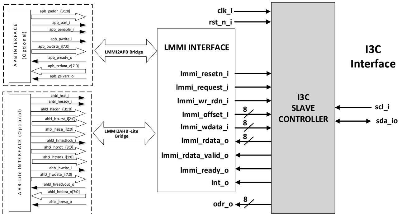
Figure 2.1. I3C Slave IP Core Functional Diagram
