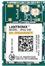
**3a.** Connect to the network using the unique xPico 240 SSID. This number refers to the last 6 digits of the serial number printed on the module. See highlighted section. The default password for this Wi-Fi Soft AP is **PASSWORD** (case sensitive).
