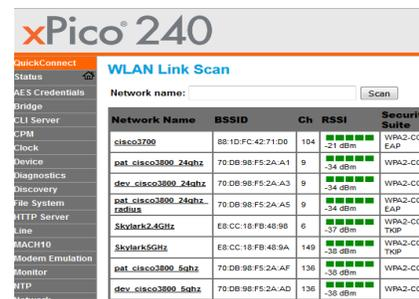
**4b.** On the Quick Connect Page, the wireless client interface can be configured. The xPico 240 can now connect to a network from the list of available wireless networks.
