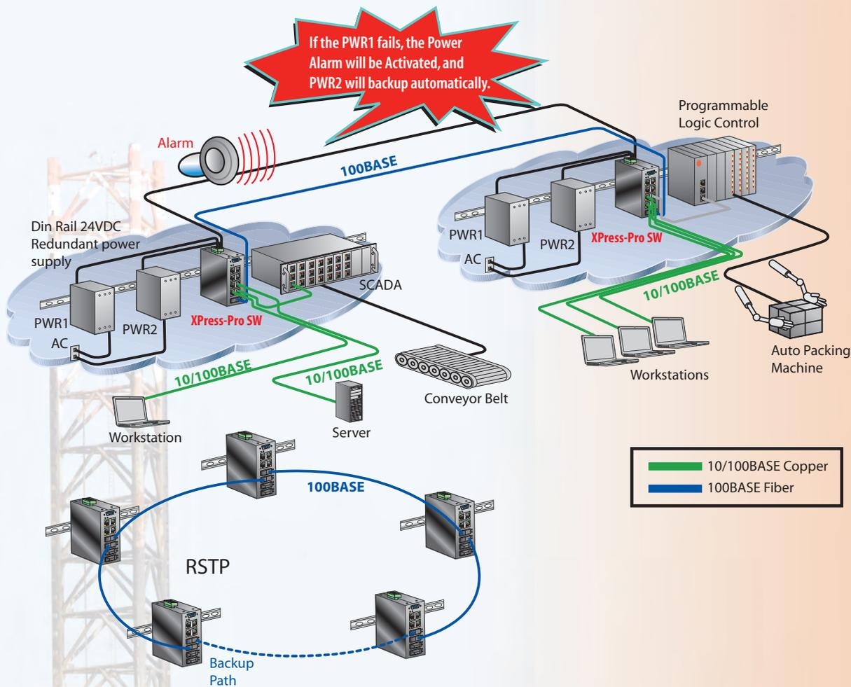
*XPress-Pro 8-port models feature redundant power inputs and a relay for power failure alarms.*
