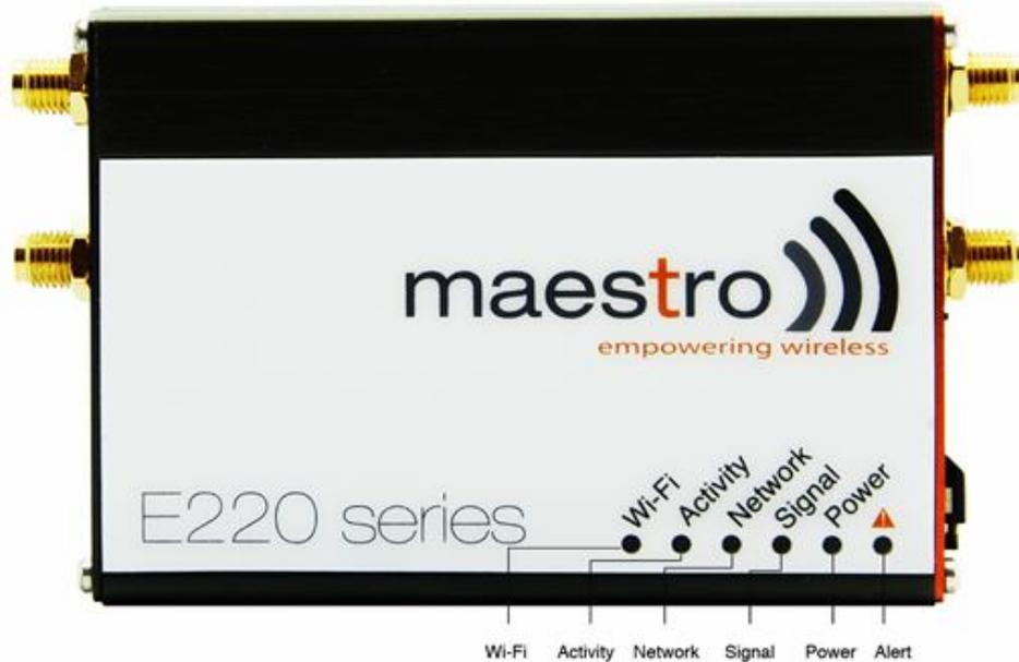
4.3.1 The top panel of Maestro's E220 Series features 6 LEDs on the front to indicate critical system information.
