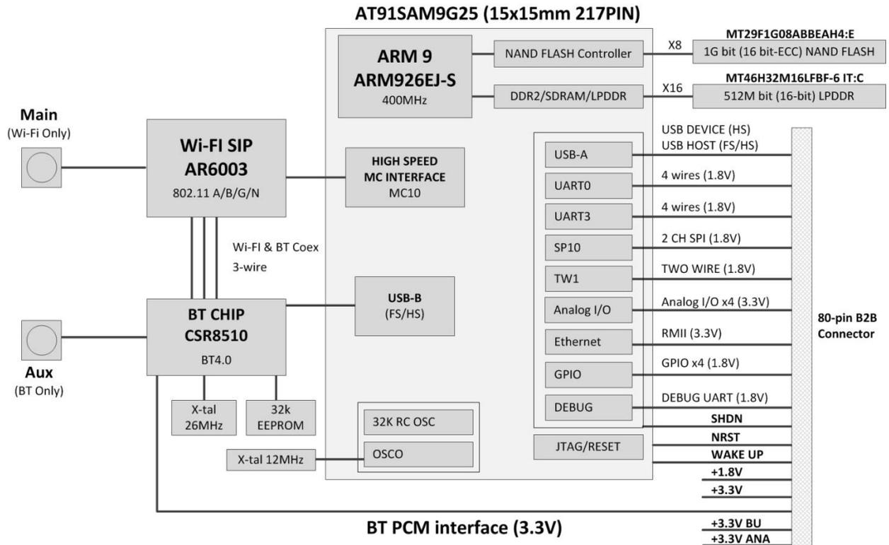
**Note:** Transmitter frequencies for Wi-Fi are 2412-2462 MHz and 5180-5805 MHz. Transmitter frequencies for Bluetooth are 2402-2480 MHz.
