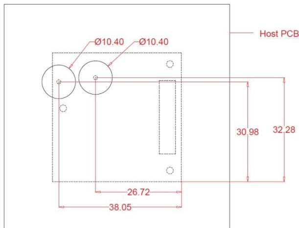
**Note:** Laird recommends that you mount the module off the edge of the board or cut out one corner and place the module in the corner to limit the cutout area. This is necessary to meet the low height requirement of the module.
