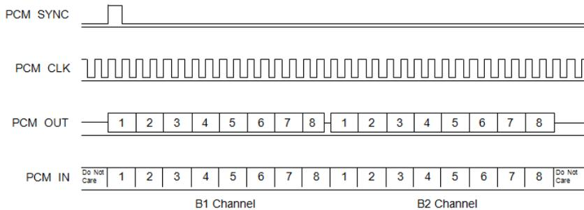
**Figure 7: Multi-slot operation**
