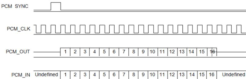
**Figure 5: Short Frame Sync (Shown with 16-bit Sample)**
