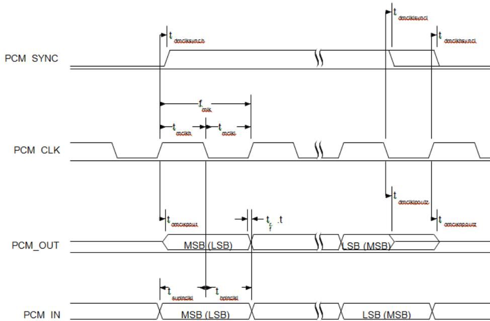
**Figure 9: PCM Master timing long frame sync**
