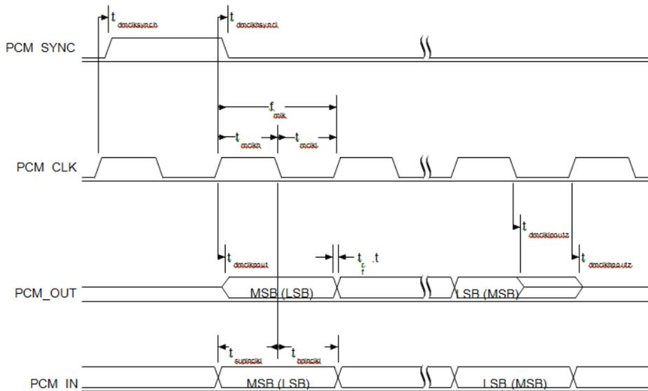
Figure 10: PCM Master timing short frame sync
