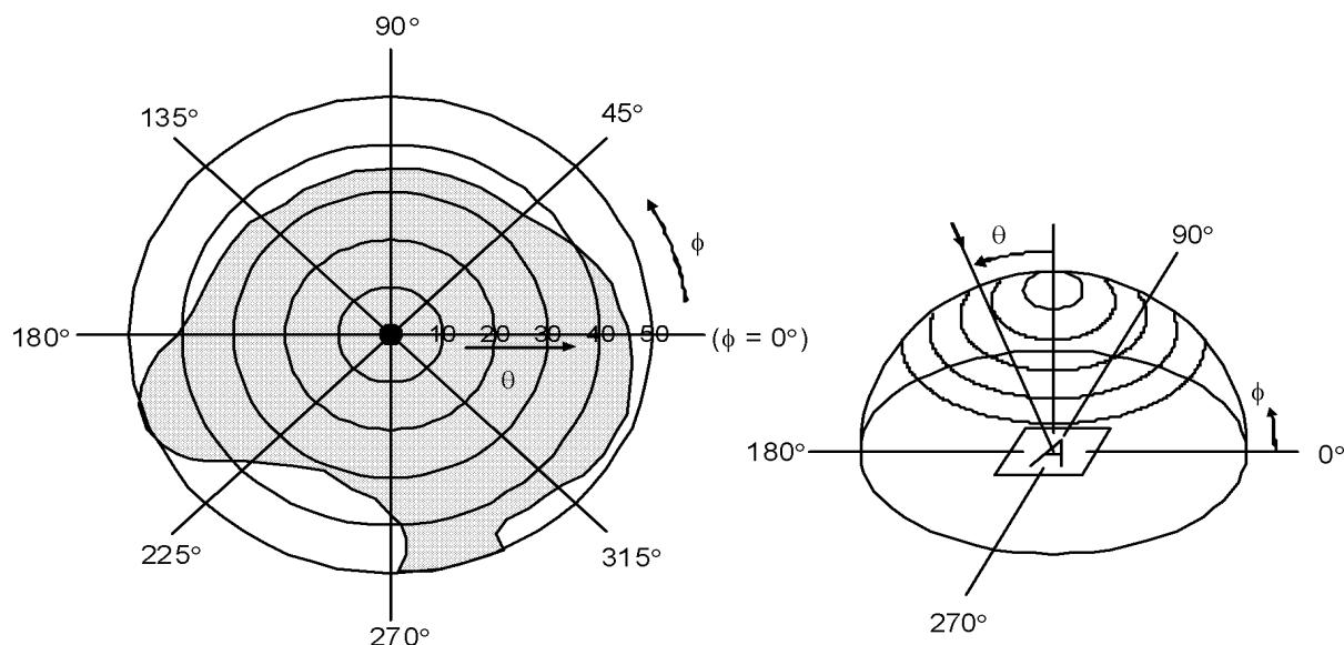
\*Area shows typ.  $CR \geq 5$  (Measuring Spot : 3.0mmφ)
