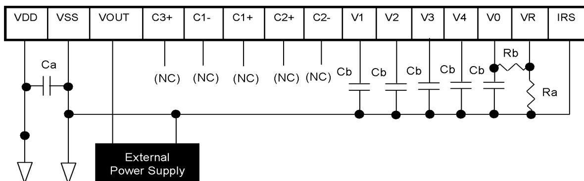
Ca : 1.0 to 4.7uF (Voltage rating 定格電圧: 10 to 35V)
