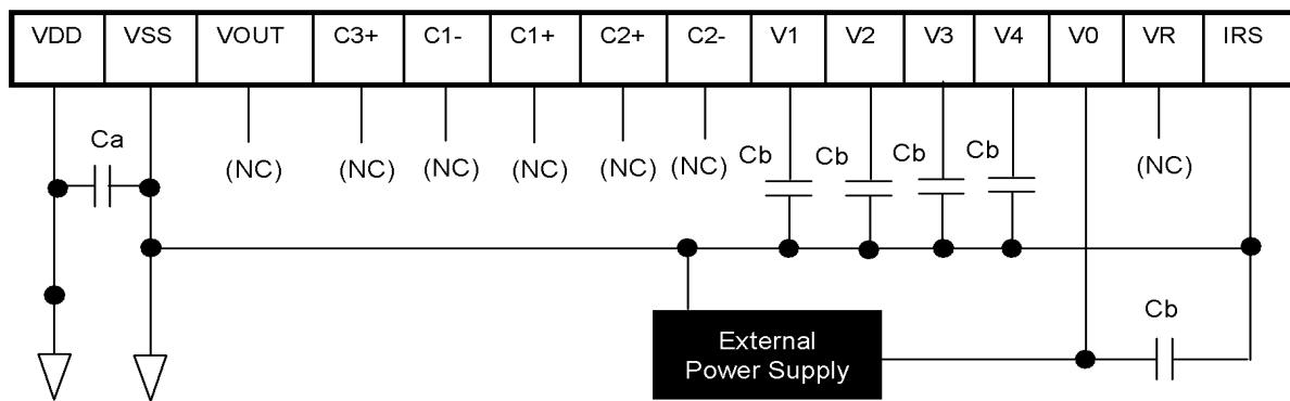
**4.2.4. When using the external power supply circuit**
