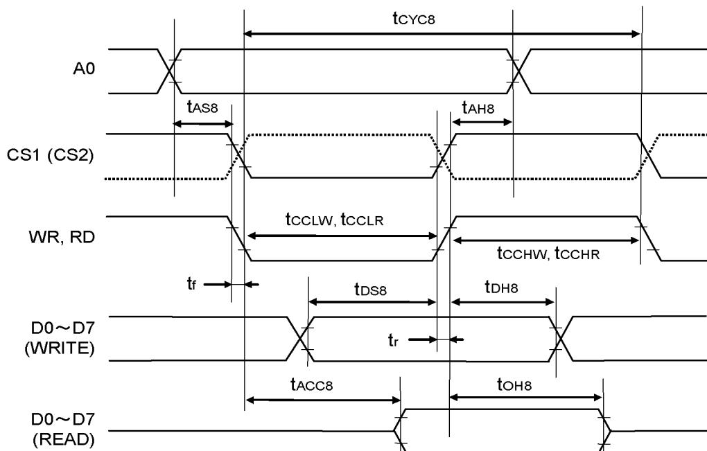
2.4.2.System Buses Read/Write Characteristics (68 series CPU)
