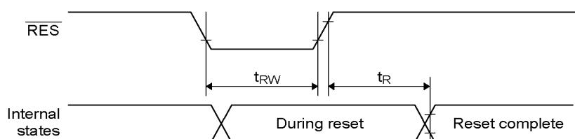
Note : The input signal rise time and fall time ( $t_r$ ,  $t_f$ ) is specified as 15ns or less.
