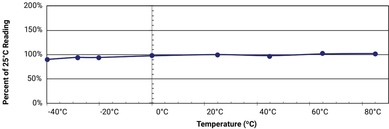
**LEAKAGE CURRENT VS. TEMPERATURE**
