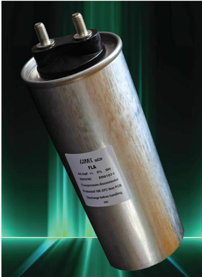
The FLA series uses metallized polypropylene dielectric, aluminum can, impregnated with soft PU specially treated to have a very high dielectric strength in operating conditions up to 85°C.
