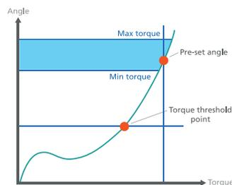
This mode gives priority to the angle to be reached. Starting from the pre-set threshold torque, the system will start counting the degrees and when the pre-set angle is reached the screwdriver will stop.
