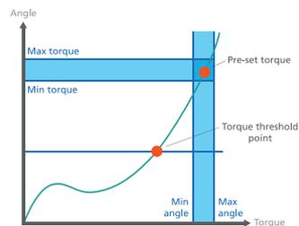
It's the most common mode. If the final torque and angle values are within the pre-set minimum and maximum values, the screw is tightened correctly and the controller will give an OK message.
