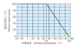
在环境温度70℃以上使用时,应按照左图负荷减轻特性曲线,减小额定功率。 For resistors operated at an ambient temperature of 70°C or above, a power rating shall be derated in accordance with the above derating curve.
