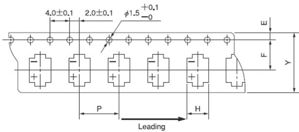
Fig. 1-2 Carrier tape  $\phi D \geq 12.5$
