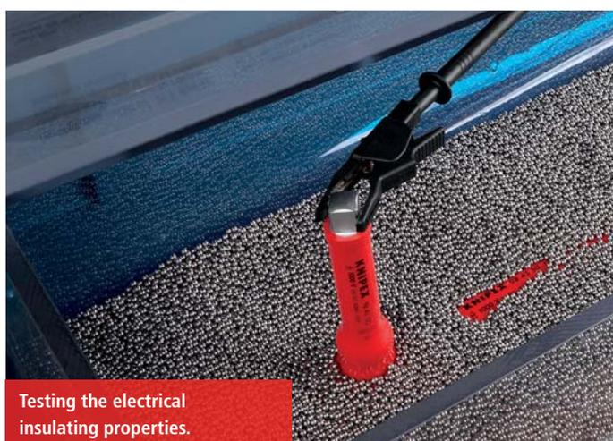
Testing the electrical insulating properties.
