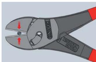
Insert the wires as close to the hinge as possible. In case of cutters with very high transmission, the width of the gap between the cutting edges close to the fulcrum may be less than the thickness of the wire. Wires may slip forward when the cutting starts.
