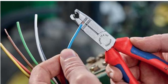
Stripping holes for conductors of 1.5 mm<sup>2</sup> and 2.5 mm<sup>2</sup>
