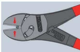
First make a notch in the wire using the KNIPEX TwinForce® until the required hand force increases considerably. Now open the pliers and slide the wire backwards towards the joint.
