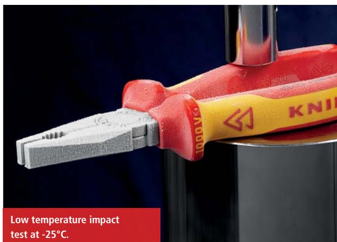
Low temperature impact test at -25°C.
