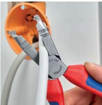
Cutting cable up to 13 mm diameter
