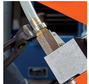
Sealing the hose connection on central lubrication
