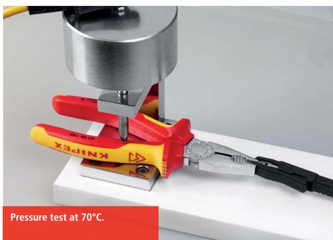
Pressure test at 70°C.
