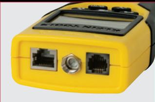
RJ45, F-Connector and RJ11/12 Jacks
