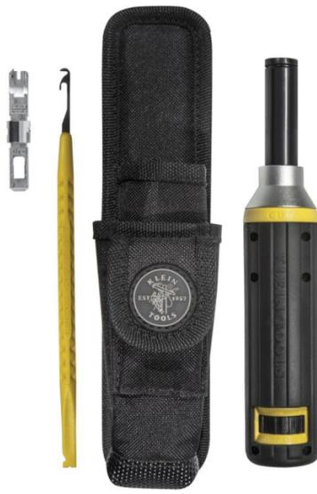
The Cushion-Grip Impact Tool Kit provides everything required to install and maintain 110 and 66 panels, cross-connect systems and wall jacks with secure terminations. Utilizing an optimized two-step impact process, the punchdown tool precisely inserts and then trims off excess wire. The 4-Piece kit comes with punchdown tool, wire pick, blade and pouch.
