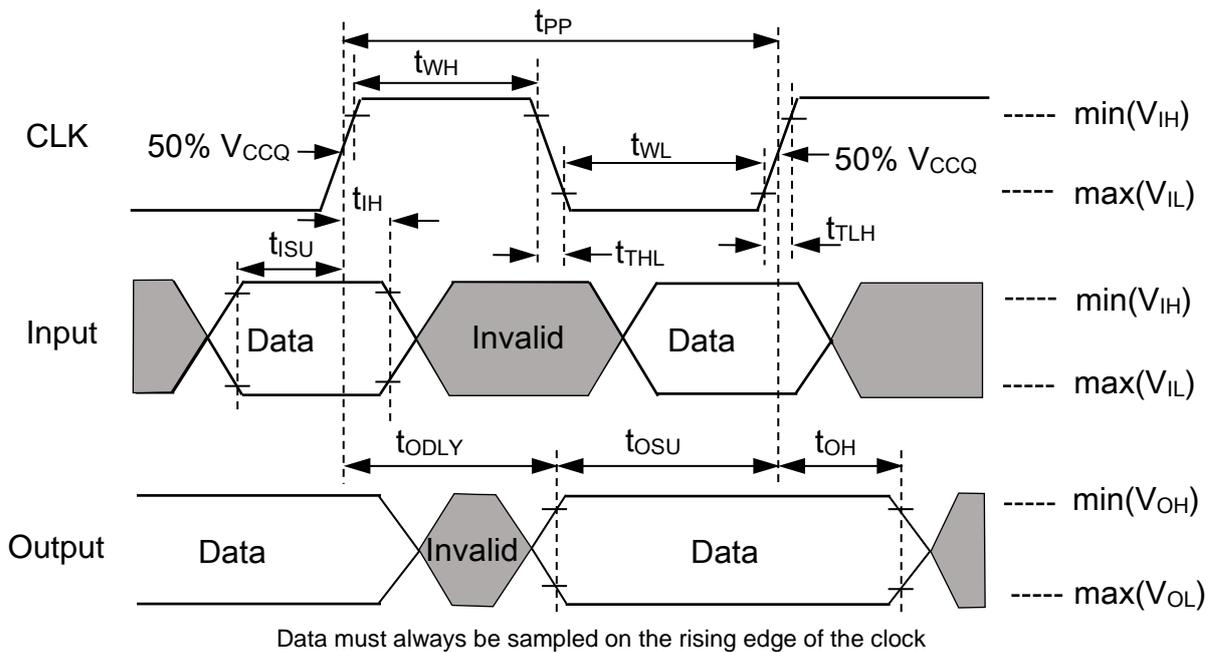
**Device Interface Timings (High-speed interface timing)**
