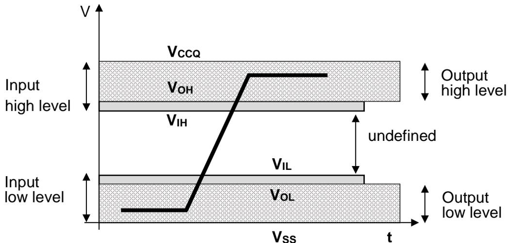
**Open-Drain Mode Bus Signal Level**
