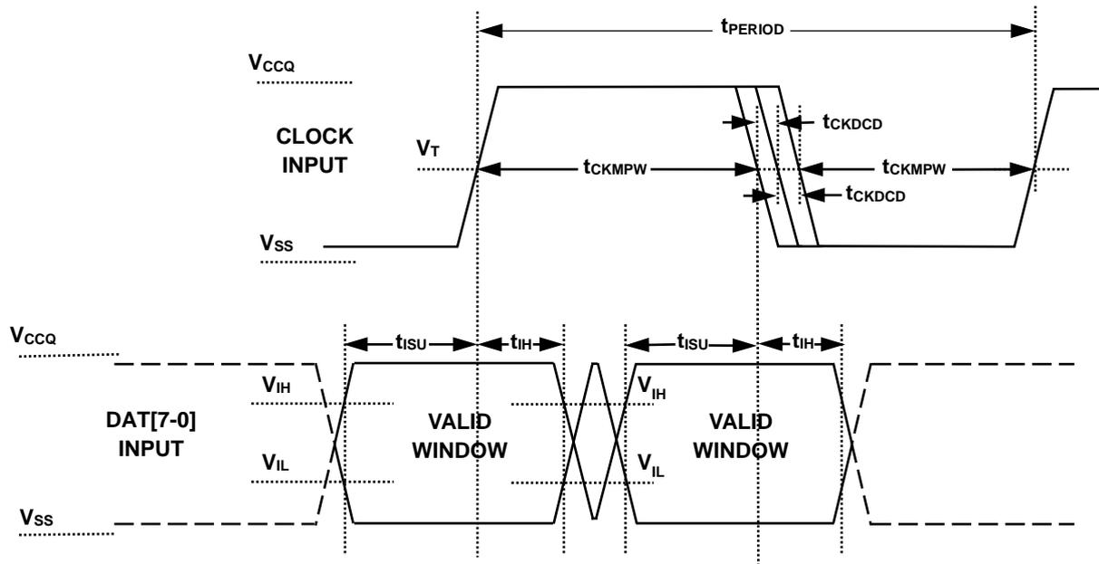
Note: V<sub>T</sub> = 50% of V<sub>CCQ</sub>, indicates clock reference point for timing measurements.
