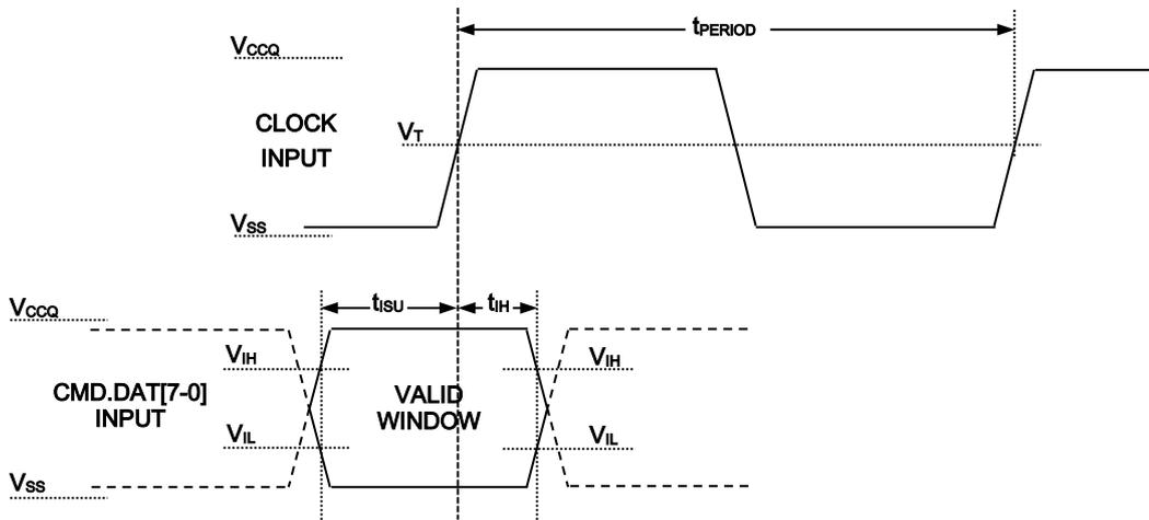
Note 1:  $t_{ISU}$  and  $t_{IH}$  are measured at  $V_{IL(max.)}$  and  $V_{IH(min.)}$ .
