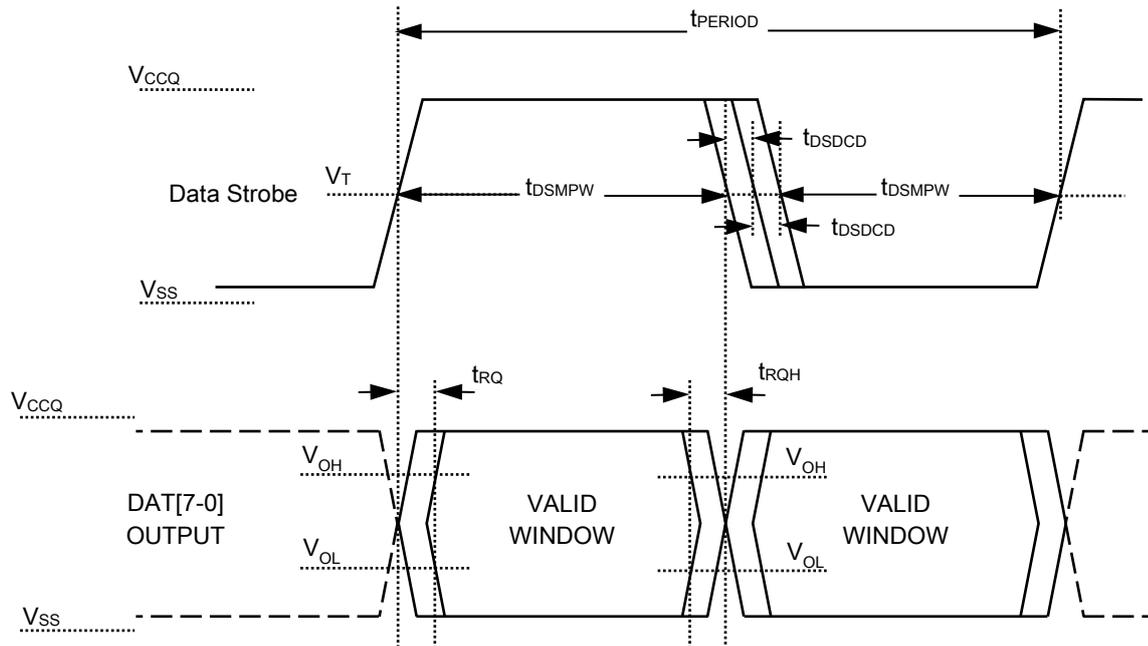
Note: V<sub>T</sub> = 50% of V<sub>CCQ</sub>, indicates clock reference point for timing measurements.
