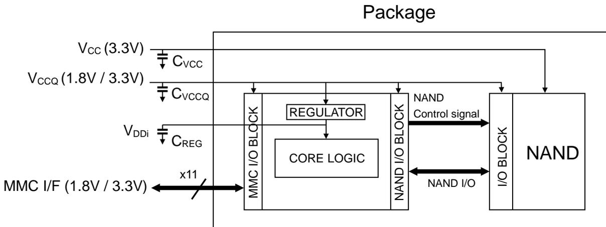
Figure 1 THGBMJG8C2LBAIL Block Diagram
