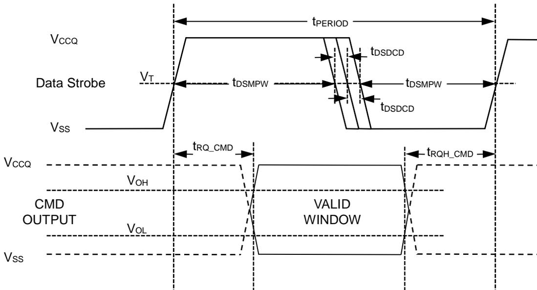
Note:  $V_T = 50\%$  of  $V_{CCQ}$ , indicates clock reference point for timing measurements.
