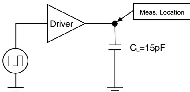
Note 1:  $C_L$  is total equivalent lumped capacitance for each Driver.
