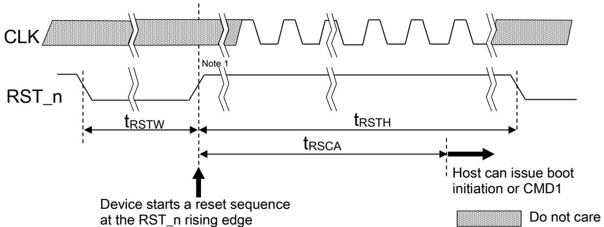
Note 1: Device will detect the rising edge of RST\_n signal to trigger internal reset sequence.
