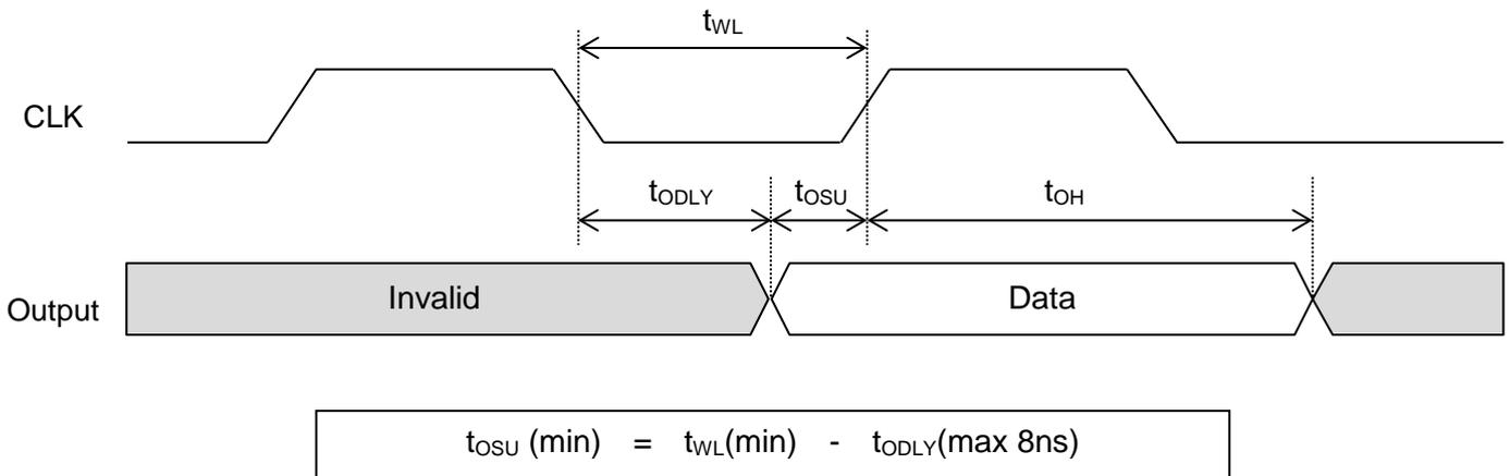
**Figure 2 Output timing**
