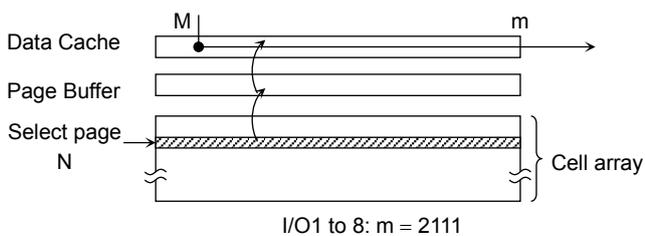
A data transfer operation from the cell array to the Data Cache via Page Buffer starts on the rising edge of  $\overline{WE}$  in the 30h command input cycle (after the address information has been latched). The device will be in the Busy state during this transfer period.
