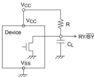
This data may vary from device to device. We recommend that you use this data as a reference when selecting a resistor value.
