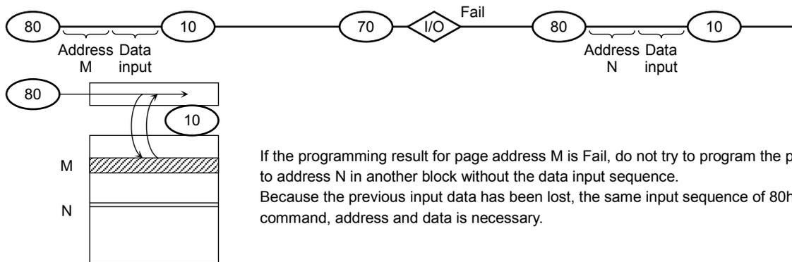
If the programming result for page address M is Fail, do not try to program the page to address N in another block without the data input sequence. Because the previous input data has been lost, the same input sequence of 80h command, address and data is necessary.
