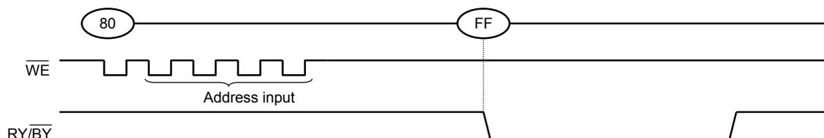
If a command other than "85h", "10h" or "FFh" is input, the Program operation is not performed and the device operation is set to the mode which the input command specifies.
