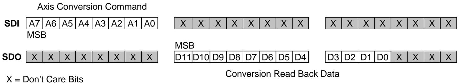
Figure 6 Register Diagram for 12-Bit ADC Read Operation
