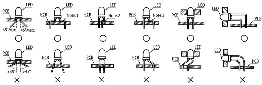
Note 1-3: Do not route PCB trace in the contact area between the leadframe and the PCB to prevent short-circuits.
