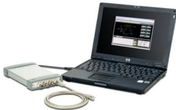
Figure 2. U2761A used as a standalone instrument
