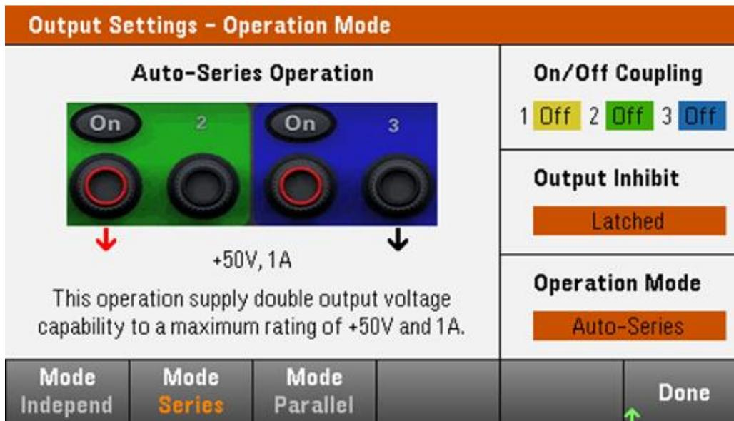
Figure 2. Auto-series operation to double the output voltage
