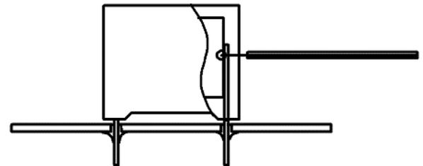
*Temperature monitored inside the capacitor.*
