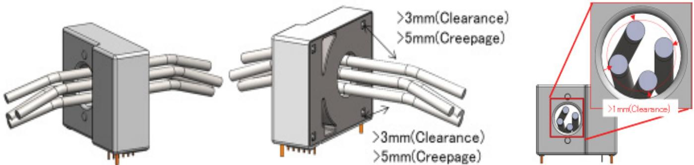
Reinforced insulation, insulation material group III, pollution degree 2, altitude < 5,000 m and overvoltage category II.
