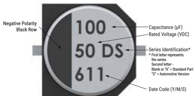
Note: 6.3 V rated voltage shall be marked as 6 V, but 6.3 V shall be assured.
