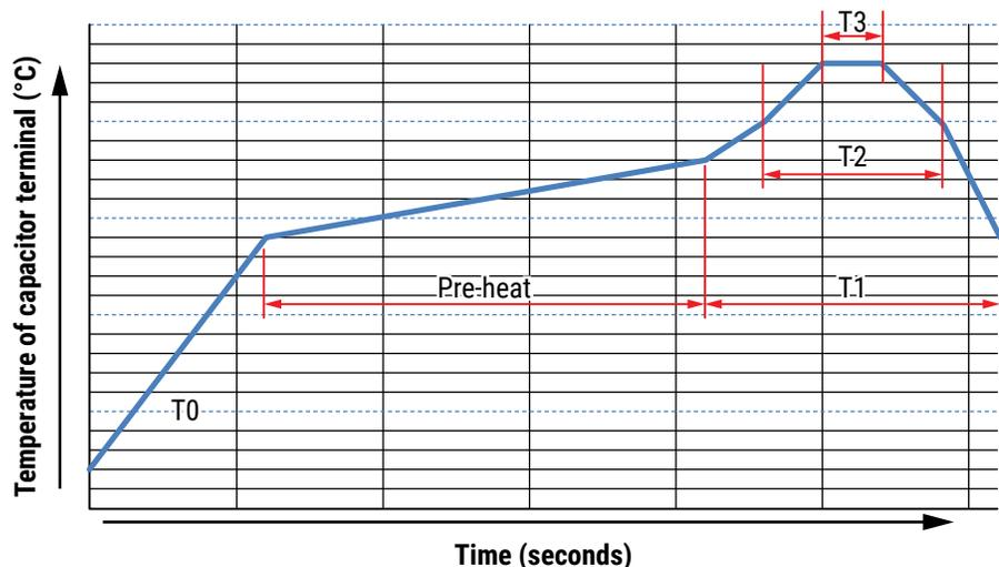
Vapor heat transfer systems are not recommended. The system should be thermal, such as infra-red radiation or hot blast
