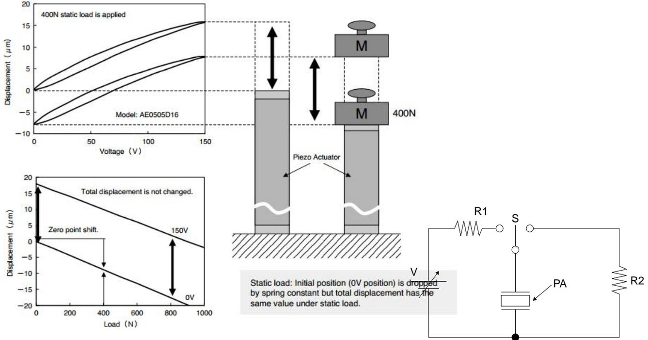
Fluctuating load: Load value changes by spring reaction when actuator moves.
