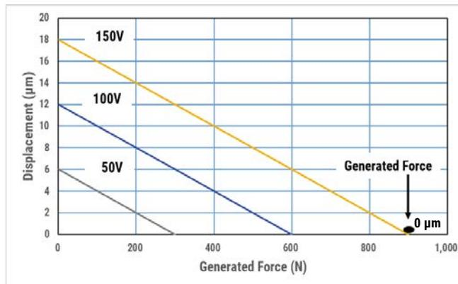
Figure 3 - Generated Force vs. Displacement - 1
