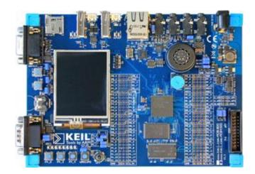
The Keil MCB1800 Evaluation Boards enable you to create and test working programs based on the NXP LPC1850 family of ARM Cortex<sup>™</sup>-M3 processor-based devices.
