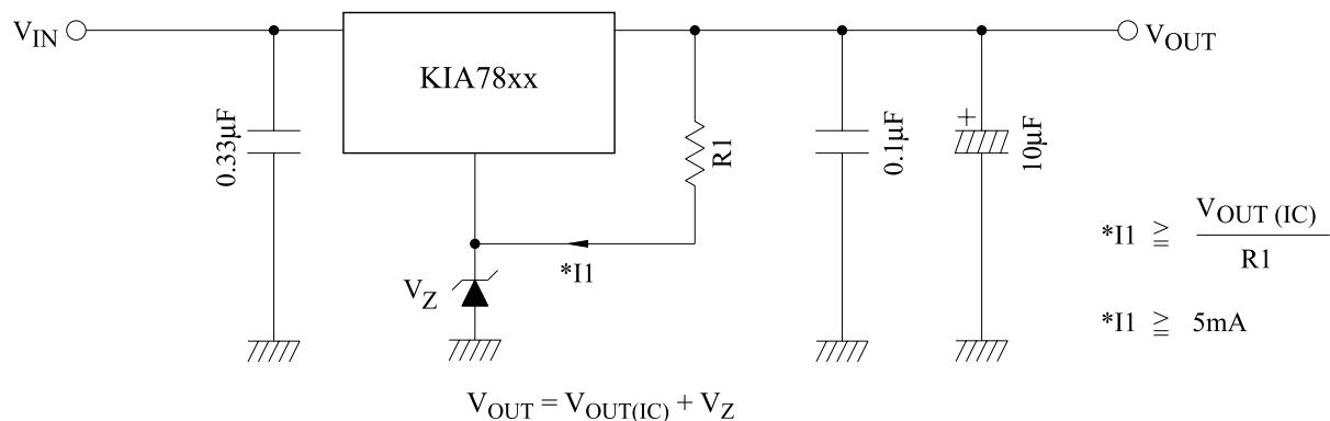
(b) Voltage boost by use of resistor
