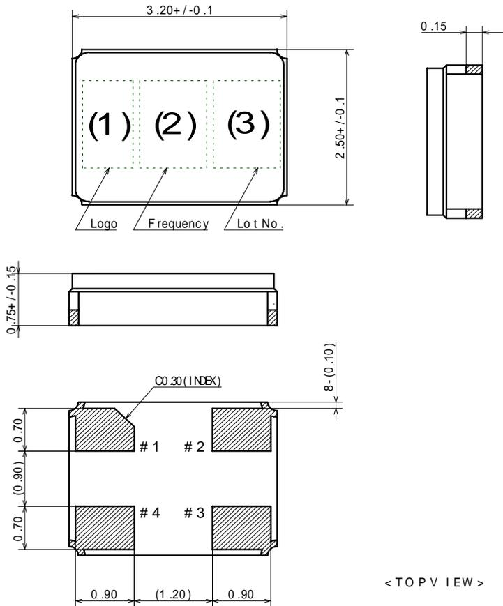
It is recommended that #2,4 is connected with GND.
