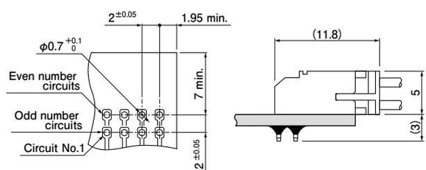
Note: 1. The above figure is the figure viewed from soldering side.
