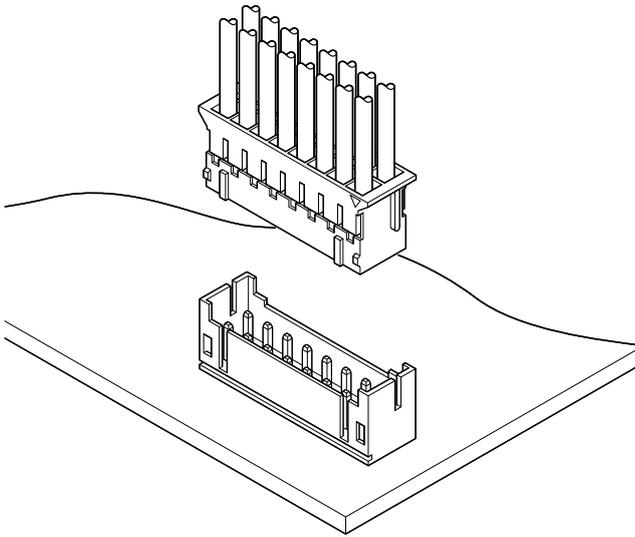
This is a 2.0 mm pitch, crimp style, dual-row, wire-to-board connector. It is designed to meet the demand for high-density and low-profile connection.
