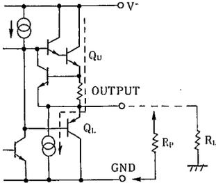
NJM2902, in its static state (No in and output condition) when design,  $Q_U$  being biased by constant current (breake down beam) yet,  $Q_L$  stays OFF.
