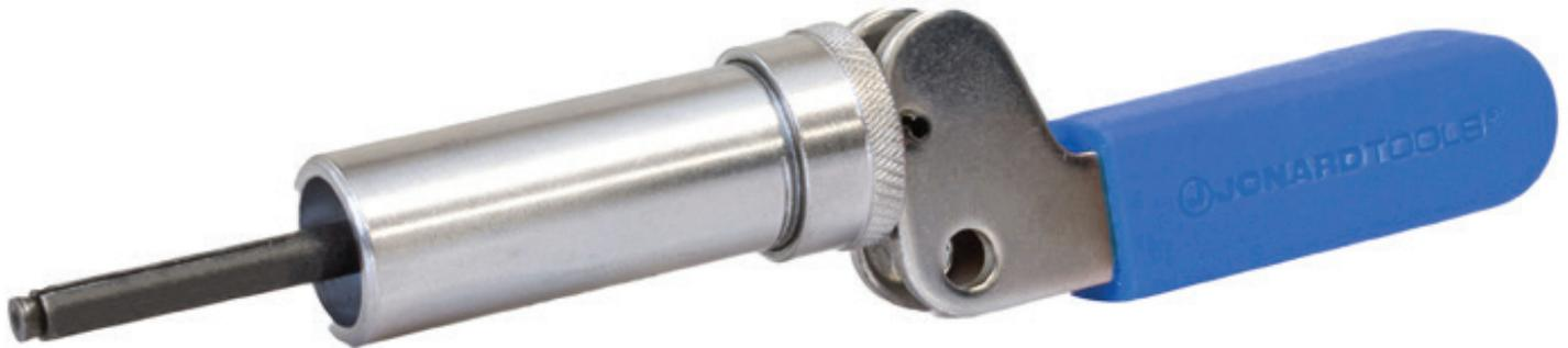
This barrel lock plunger key is the perfect tool for use on Highfield, Channell, and Innertite barrel locks with inside diameters of 0.176" to 0.196". This tool is also compatible with the Channell LK03029817, Highfield 93180775-S, and used in CATV Pedestal Applications. This barrel lock plunger features the following:
