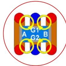
Mutual coupling from opposing polarity vias lowers inductance when mounted on a PCB.
