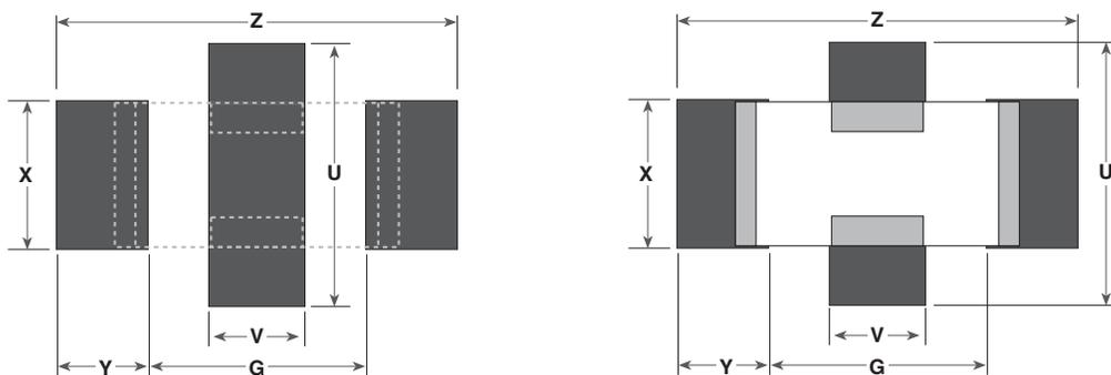
Use of solder mask beneath component is not recommended.
