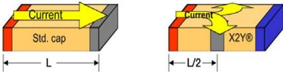
The X2Y® has short, multiple and opposing current paths resulting in lower device inductance.
