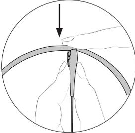
Insert the cable into the cable collector clip. Do not leave the cable longer than necessary to reach the work area freely.
