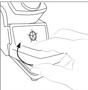
Lift the wiper at its front edge.
