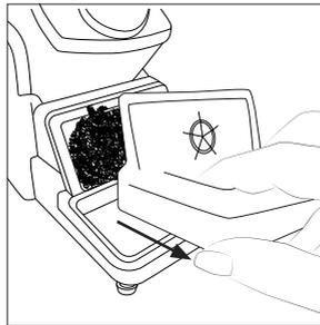
Remove the wiper by pulling it out.
