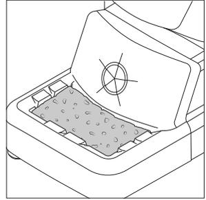
The softest cleaning method. Keep the sponge damp with distilled water when working to avoid tip wear.
