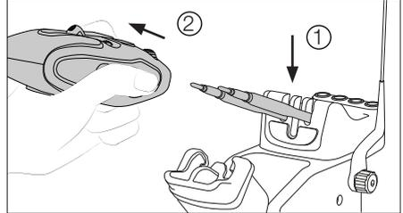
Place the cartridges in the extractor (1) and pull the tweezers to remove them (2).
