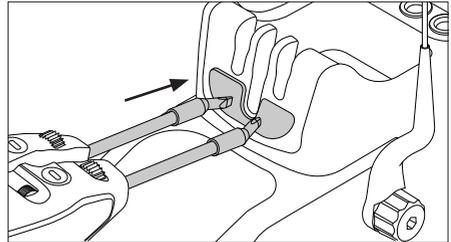
Press the cartridges against the extractor and make sure that the cartridge are inserted up to the mark\*.
