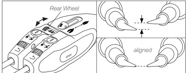
The wheel allows the tips to be adjusted so that they are aligned when the tweezers are closed.
