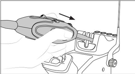
Use the vertical grooves to position the cartridges and place the tweezers onto the cartridges.
