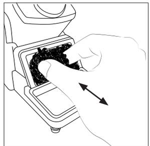
Replace the brass wool with a new one when it is worn out. Place the wiper back or replace them if desired.
