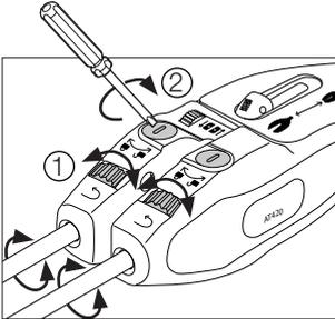
Slightly turn the wheels to align the cartridges as required (1). Then lock the cartridge fixing screws\* (2).
