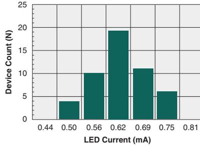
**Typical  $I_F$  for Switch Dropout**
