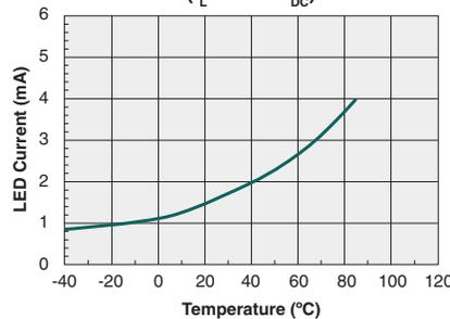
**Typical  $I_F$  for Switch Dropout vs. Temperature**
