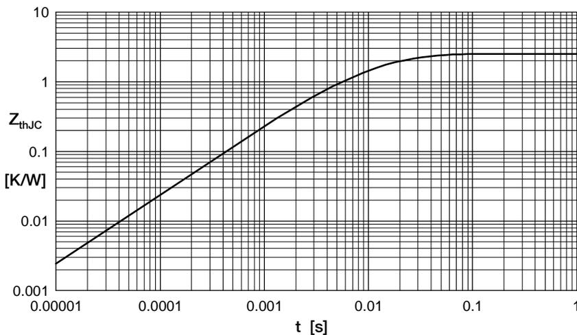
Fig. 7 Transient thermal impedance junction to case
