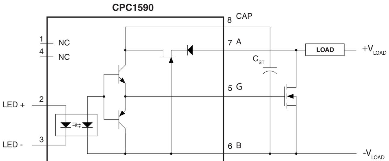
between 10V and 16V. The capacitor's voltage rating should be two to three times this range.
