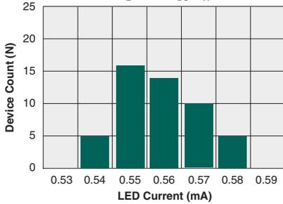
**Typical  $I_F$  for Switch Dropout**
