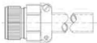
AF CLASS..... Short backshell, with A style clamp and bushing. Non-environment proof.
