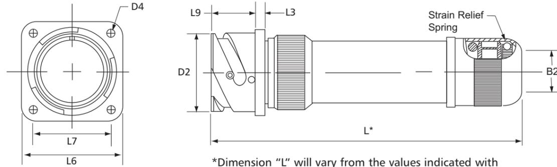
\*Dimension "L" will vary from the values indicated with escalating or de-escalating backshells and some special insert configurations. Verify with our Customer Service Department.
