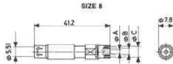
Coaxial contacts in this table are used in Size "8" contact cavities of F80 inserts. For electrical characteristics please consult the factory.
