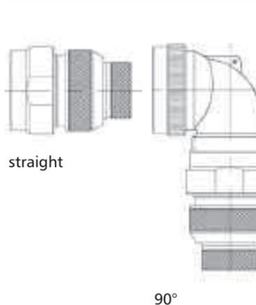
SBT CLASS.... Similar to SB but the backshell includes a knurled extension for the shield termination via tincl lock ring (not supplied). Environment proof.
