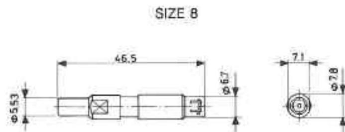
Male - female coaxial contacts can be used on the CIR-TB connectors with inserts having size "8" contact cavities. Inserts are F80 type. To be mated with all "C8" types that are independent from the cable used.
