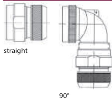
SB CLASS..... Straight or 90° backshell with the swivel coupling nut and adapter suitable for use with heat shrink tubing or boot. The shield is terminated and secured with the wire prior to tightening the backnut. Wire sealing grommet is included. Recommended to use with RFI fingers in CIRG06SB/CIRG08SB. Environment proof.
