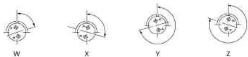
Alternate Positions of Insert Arrangements (Key Stationary - Insert Rotated)
