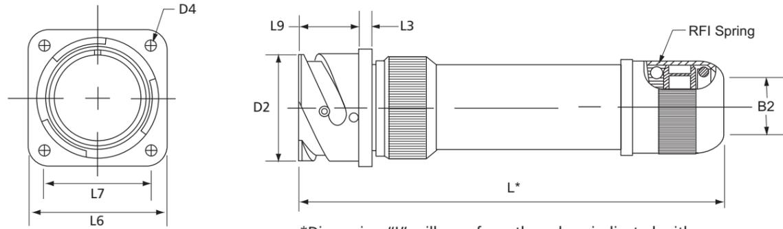
\*Dimension "L" will vary from the values indicated with escalating or de-escalating backshells and some special insert configurations. Verify with our Customer Service Department.
