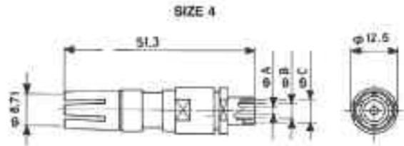
Coaxial contacts in this table are used in Size "4" contact cavities of F80 inserts. For electrical characteristics please consult the factory.
