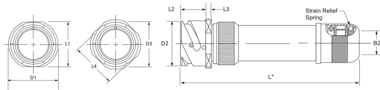
\*Dimension "L" will vary from the values indicated with escalating or de-escalating backshells and some special insert configurations. Verify with our Customer Service Department.
