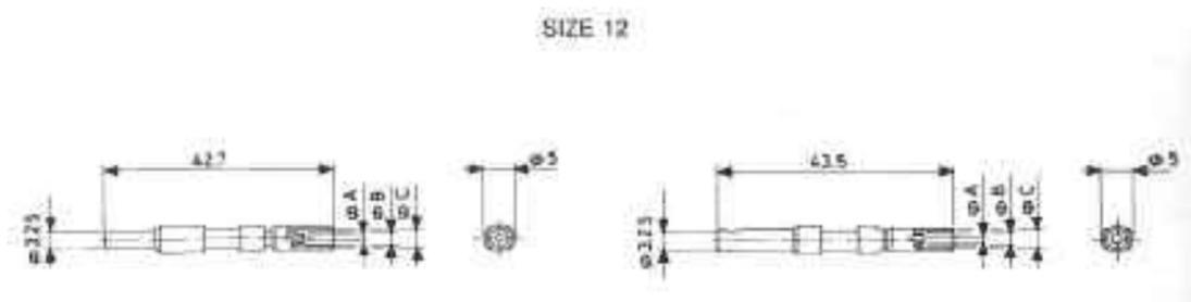
Coaxial contact in the table below are used in Size "12" contact cavities of F80 inserts. For electrical characteristics please consult factory.
