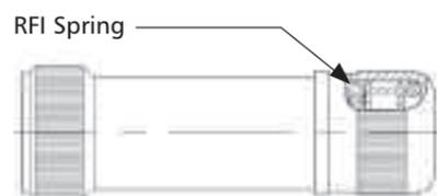
WK1 CLASS... Long WK backshell, grommet and backnut assembly suitable for shield termination and strain relief of jacket. Environment proof. Refer to page 108 for receptacle dimensions. Refer to page 152 for plug dimensions.
