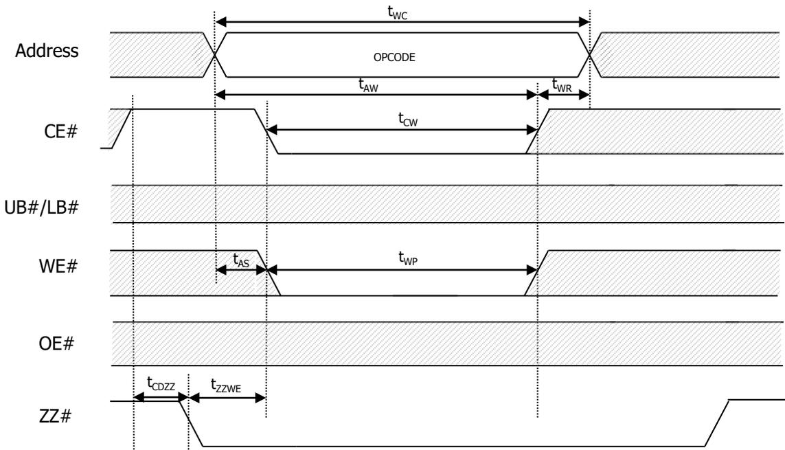
**Figure 12: DPD Entry and Exit Timing**
