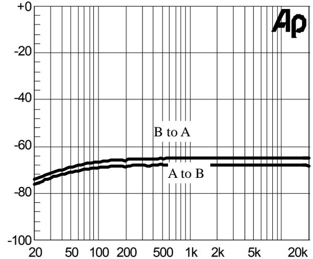
**Figure 29** Crosstalk SE mode, 3V, 320Ohm, Po=30mW
