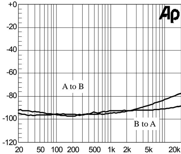
**Figure 26** Crosstalk BTL mode, 5V, 80Ohm, Po=1W
