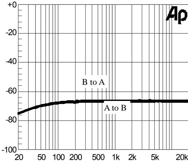
**Figure 28** Crosstalk SE mode, 5V, 320Ohm, Po=80mW
