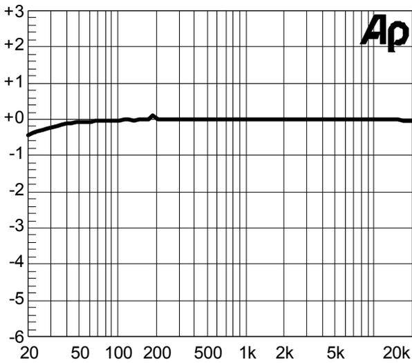
**Figure 22** Frequency Response BTL mode, 5V, 80Ohm
