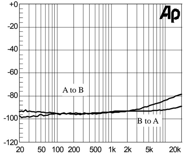
**Figure 27** Crosstalk BTL mode, 3V, 80Ohm, Po=0.3W
