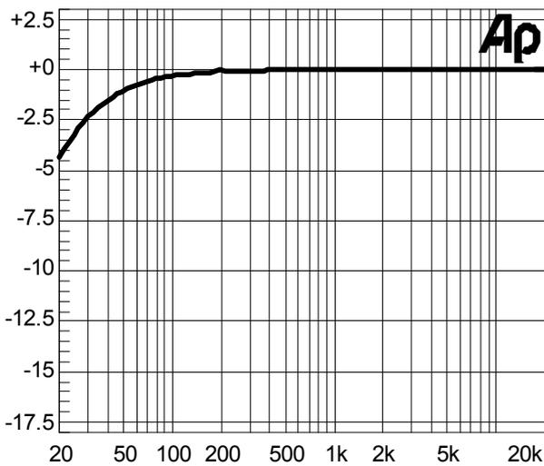
**Figure 24** Frequency Response SE mode, 5V, 32Ohm, C5/C6=220uF
