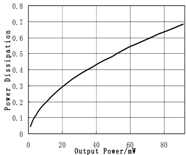
**Figure 31** Power Dissipation vs. Output Power SE mode, 5V, f=1 kHz, RL=320Ohm
