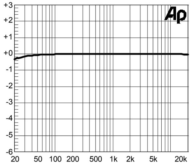
**Figure 23** Frequency Response BTL mode, 3V, 80Ohm
