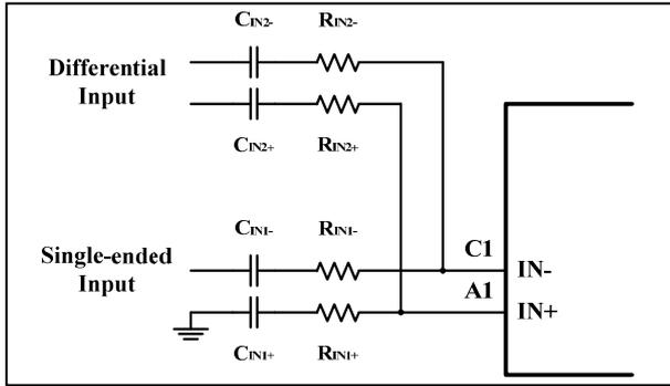
**Figure 13** Summing Differential Input and Single-Ended Input Signals
