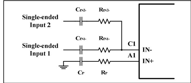
**Figure 14** Summing Two Single-Ended Inputs
