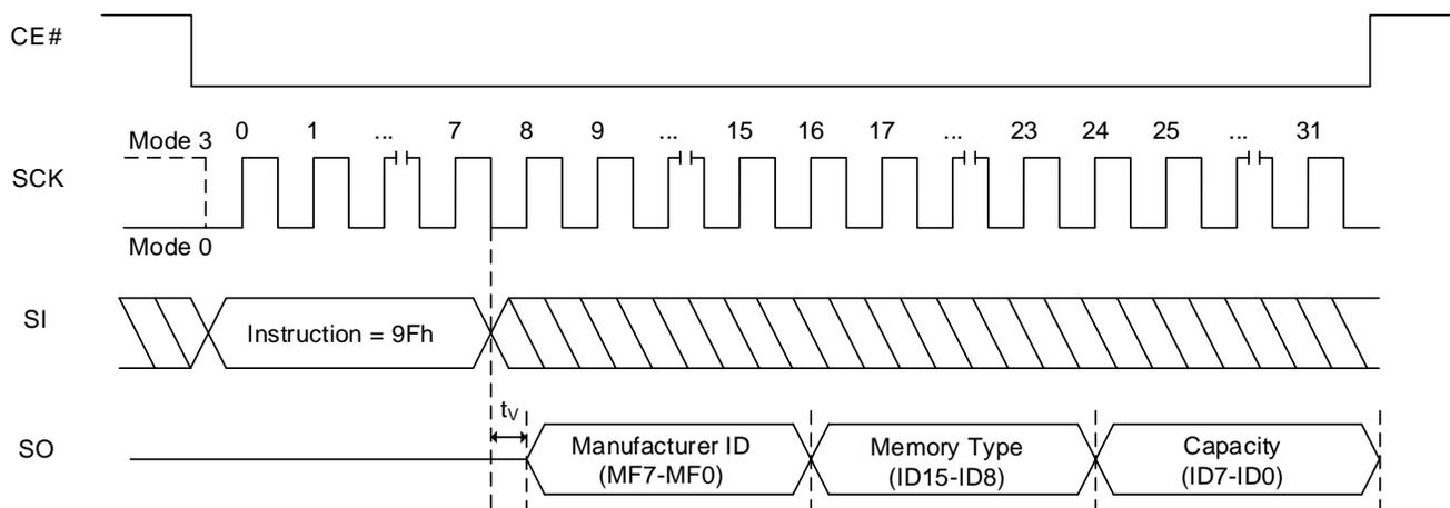
**Figure 8.53 RDJDIDQ (Read JEDEC ID In QPI Mode) Sequence**
