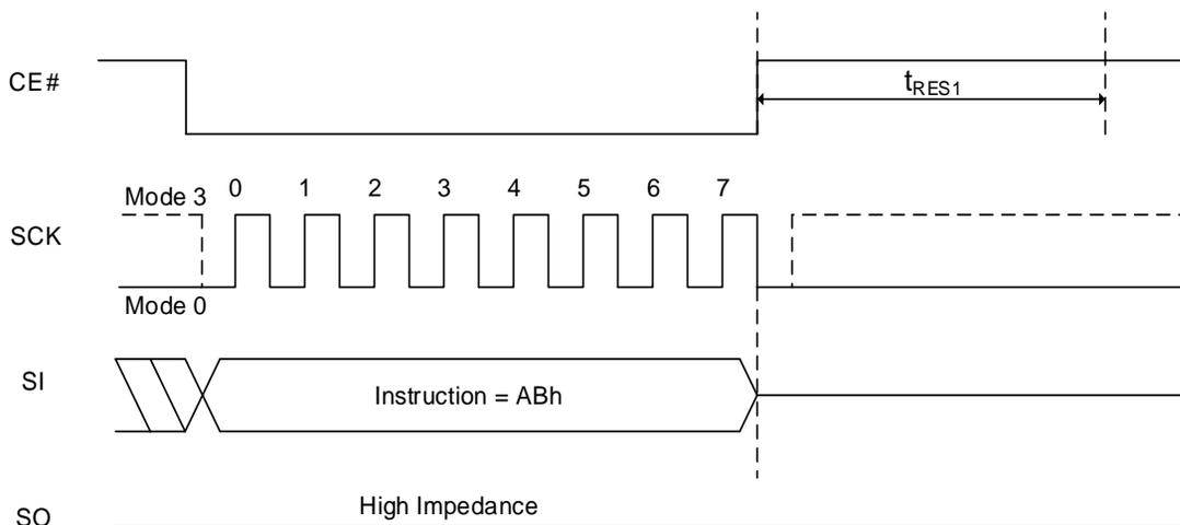
**Figure 8.39 Release Deep Power Down Mode Sequence In QPI Mode**
