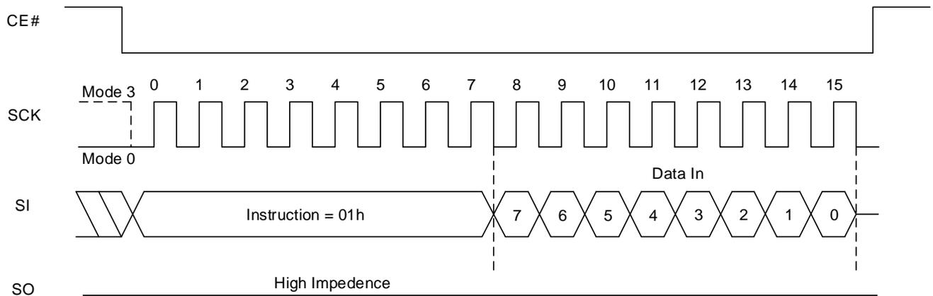
**Figure 8.29 Write Status Register Sequence In QPI Mode**
