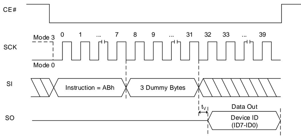
Figure 8.51 RDID (Read Product Identification) Sequence In QPI Mode
