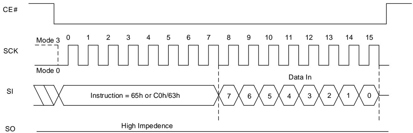
**Figure 8.41 Set Read Parameters Sequence In QPI Mode**
