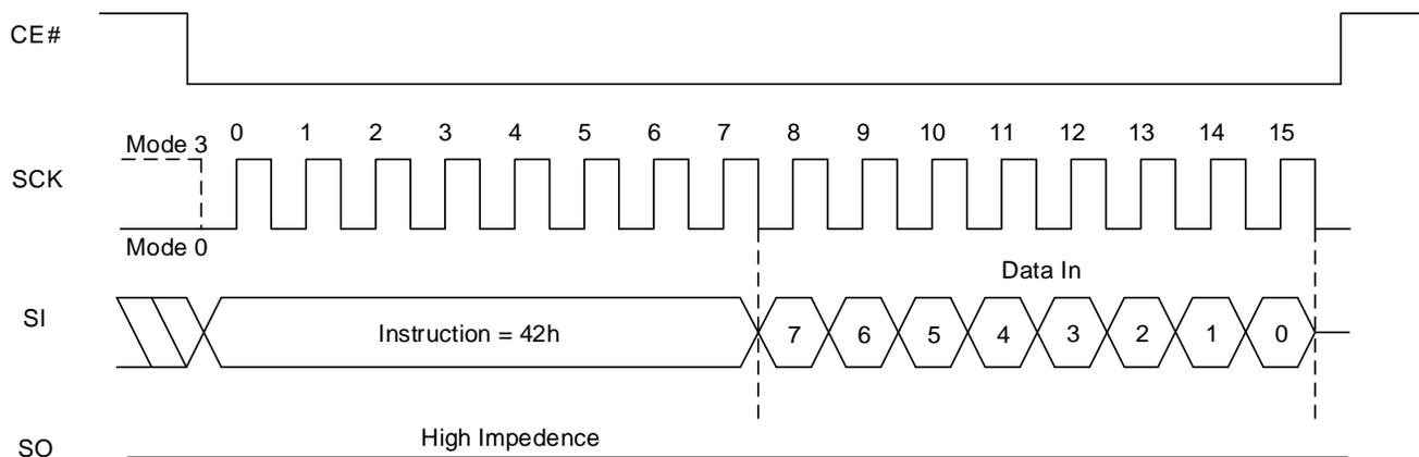
**Figure 8.33 Write Function Register QPI Sequence In QPI Mode**
