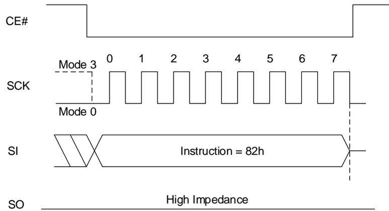
**Figure 8.49 Clear Extended Read Parameters Sequence In QPI Mode**
