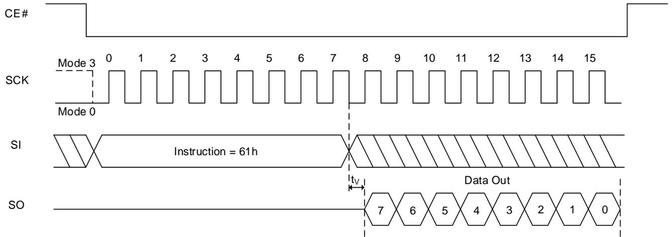
**Figure 8.45 Read Read Parameters Sequence In QPI Mode**
