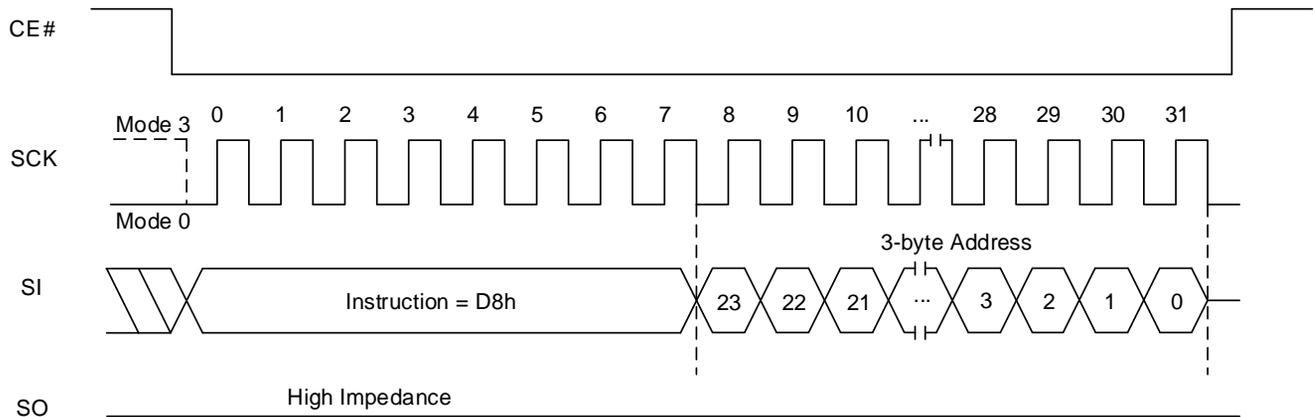
**Figure 8.17 Block Erase (64K) Sequence In QPI Mode**
