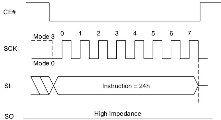
**Figure 8.73 Sector Lock QPI Sequence In QPI Mode**
