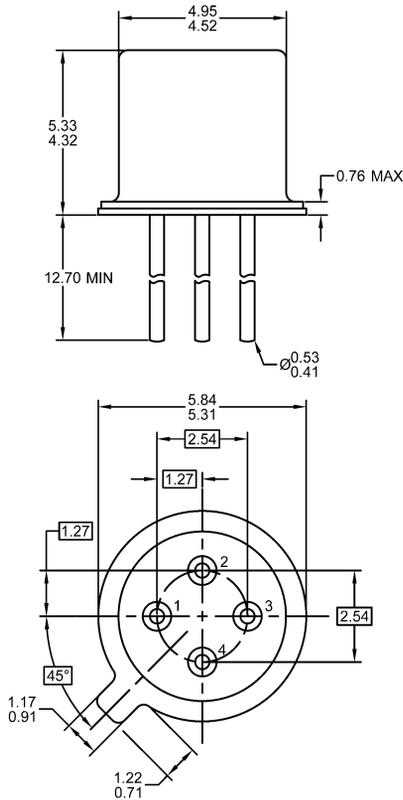
1. All linear dimensions are in millimeters.
