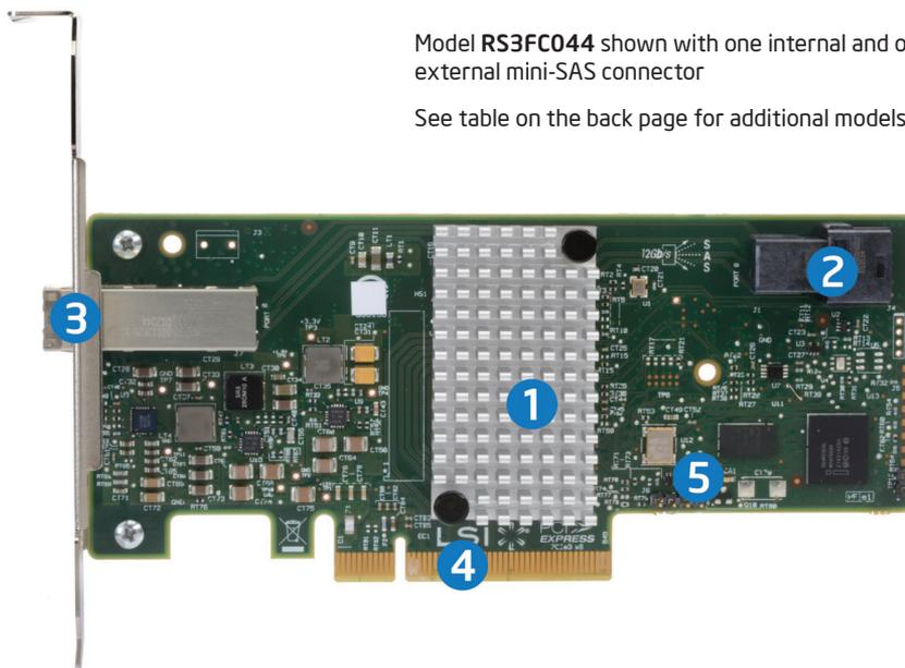
Model **RS3FC044** shown with one internal and one external mini-SAS connector
