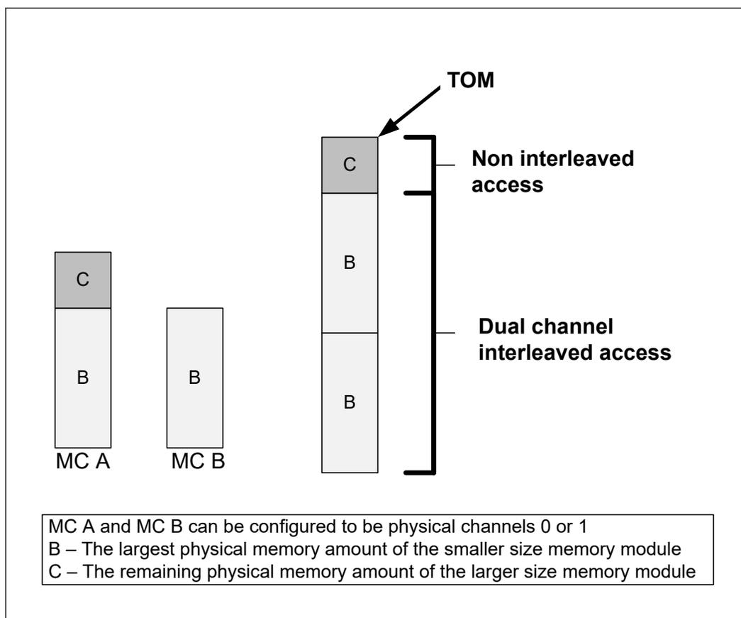
**Dual-Channel Symmetric Mode (Interleaved Mode)**
