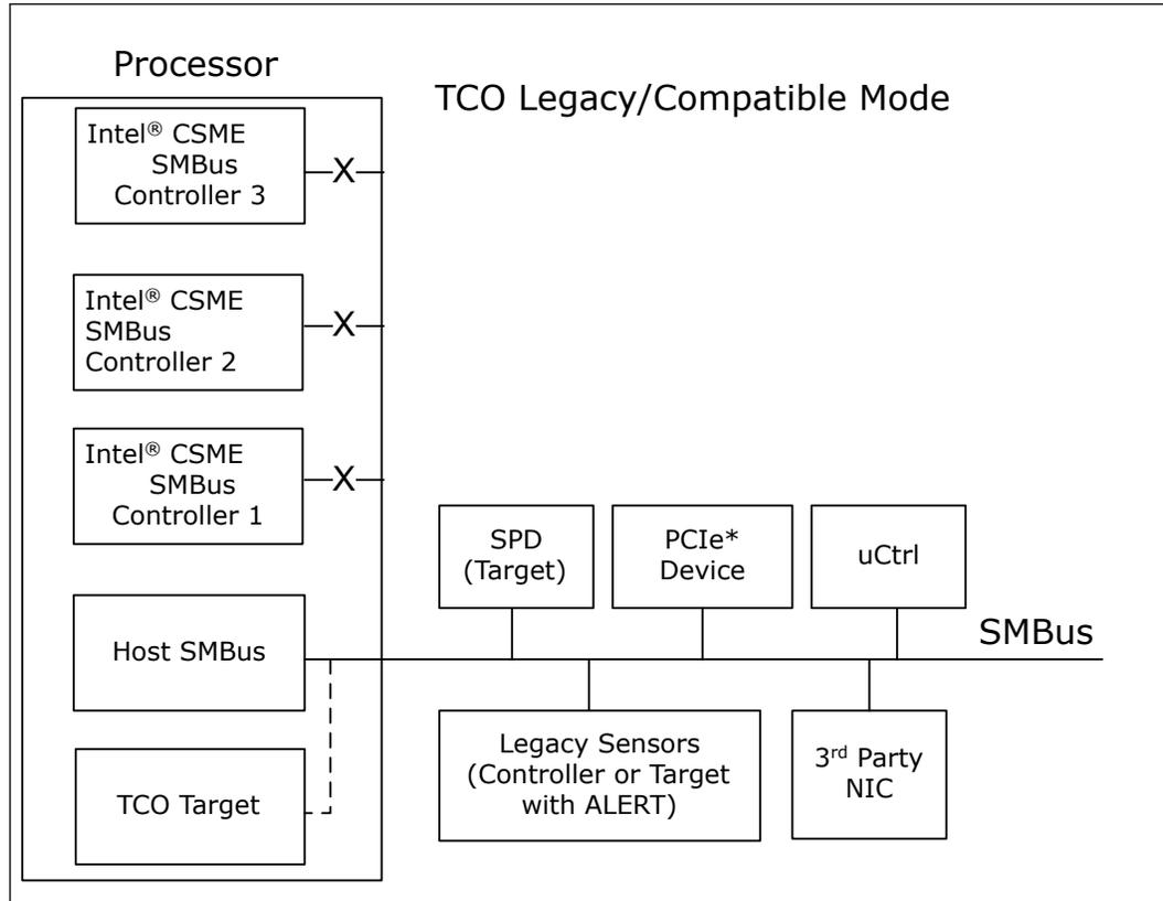
In TCO Legacy/Compatible mode the Processor can function directly with an external LAN controller or equivalent external LAN controller to report messages to a network management console. The table below includes a list of events that will report messages to the network management console.
