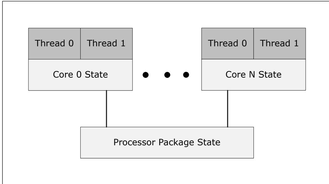
While individual threads can request low-power C-states, power saving actions only take place once the processor IA core C-state is resolved. processor IA core C-states are automatically resolved by the processor. For thread and processor IA core C-states, a transition to and from C0 state is required before entering any other C-state.
