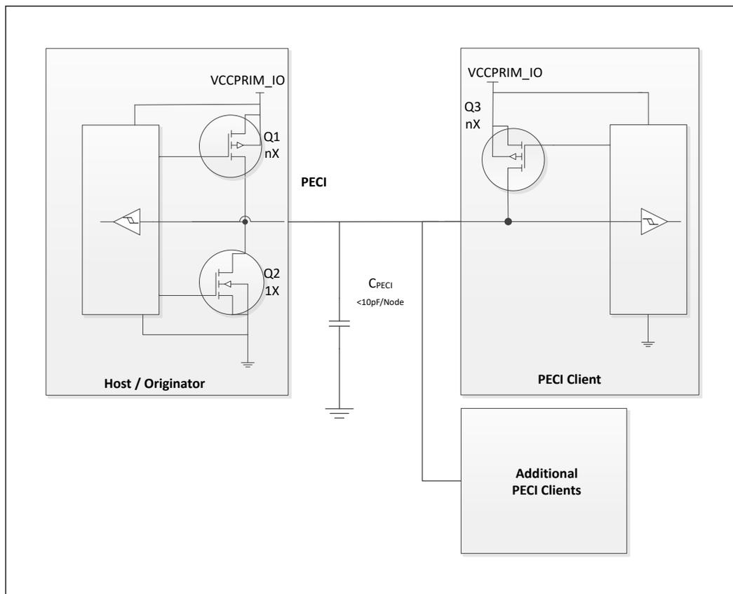
Figure 8. PEFI EC Connection Example
